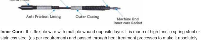
vibration free. Outer Casing: It is flexible, double interlocked, circular rounded, made of galvanized steel strip, Special spring steel lining is provided within outer casing to avoid any friction between inner core & outer casing. Connection: One end of shaft with machine end socket is attached to suitable motor and other end is
